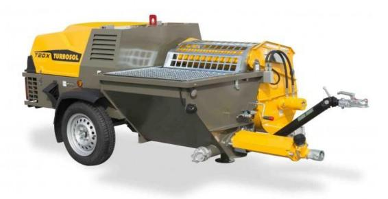
T20X is a state-of-the-art plastering machine equipped with a worm pump, lifting mixer, and closed-loop hydraulic circuit for mixing, pumping, spraying and injecting common, ready-mixed, insulating and special mortars.
