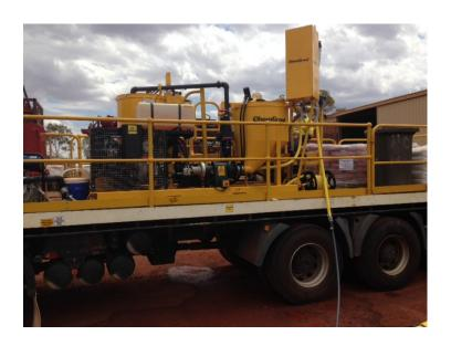
Timing for this project was critical and the notice period short with 3 weeks to commission a Mine Spec Colloidal mixers supplied and fitted to a MAN TGS 8X8 Mine Spec Truck. The MAN vehicle required significant vehicle fabrication to ensure guarding around the truck mounted mixer was to Rio Tinto safety standards. Being a mobile setup allowed Ranger to easily relocate the grout plant around the site in conjunction with the pallet of bentonite stored at the rear of the vehicle.
