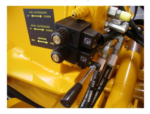
AGITATOR CONTROL controls agitator ON/OFF and FORWARD REVERSE functions.
