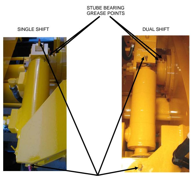
**BELL CRANK AND SHIFT** CYLINDER GREASE POINTS
