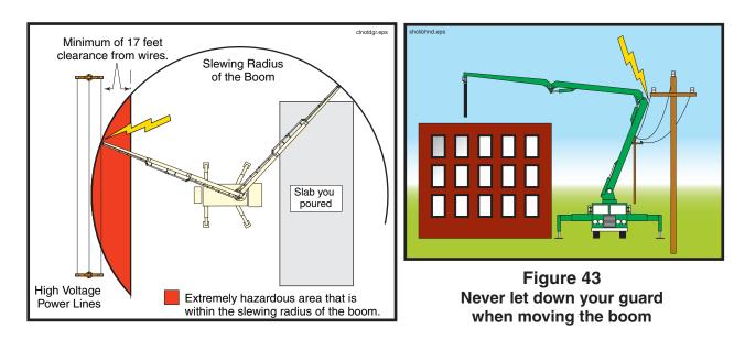
A DANGER High voltage makes conductors out of materials that would normally not conduct! Many nonconductors will conduct enough current to kill you if you contact the 8000 volts to ground that is normally found on power poles in the United States (Figure 44). Voltage in the wires may be higher than 8000, especially in industrial areas.
