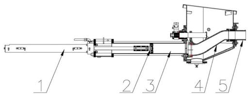
The hydraulic oil flow created by the hydraulic pump pushes the drive cylinder pistons inside the drive cylinders (1) alternately back and forth. Because the drive cylinders and concrete pistons (2) inside the concrete cylinders (3) are linked together, the pistons move synchronously.
