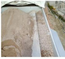
Mobile adjustable bulkhead for the sand compartment
