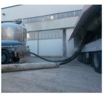
Pneumatic refilling system for cement compartment
