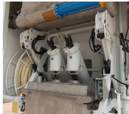
Binder silo divided into two compartments
