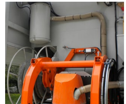
Cement powder recovery extractor fan
