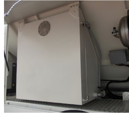
Additional water tank
