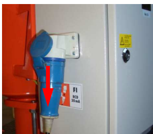
Fig. 56: Removing the connection cable
