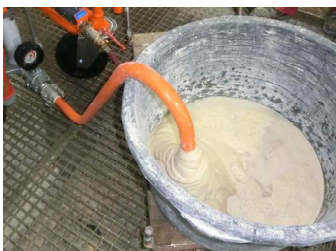
Fig. 56: Consistency of mortar
