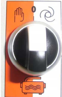
Fig. 14: Operating modes water pump
