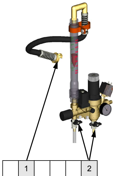
Fig. 103: Disconnect water supply
