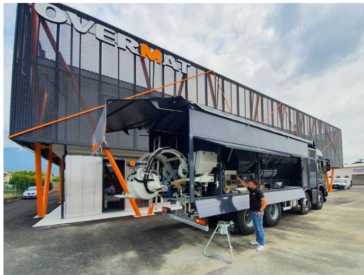
Photo: the mobile mixing barrel comes lowered to the ground for pumping
