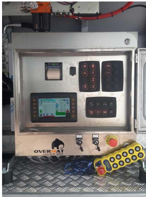
Photo: the operator panel with integrated printer and the radio control bidirectional.
