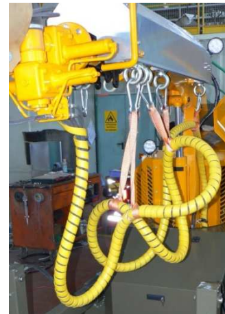
Fig. 7.5-2 - Examples of hydraulic pipes of the boom collected for movement
