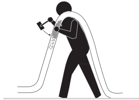
Fig. 7.11-1 - Clogging search on rubber pipe
