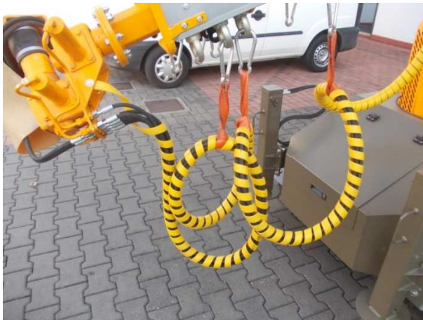
Fig. 7.5-2 - Examples of hydraulic pipes of the boom collected for movement
