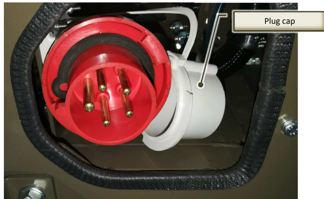
Fig. 5.6-1 - Machine electric control board supply plug
