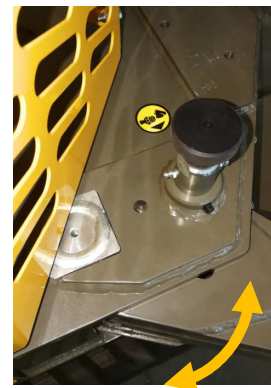
Fig. 7.6-1 - Spring positioning pin of an outrigger
