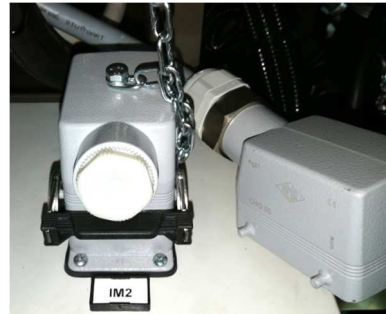
Fig. 7.4-7 - Cap in the “IM2” plug of the electric control board for machine operation without radio control
