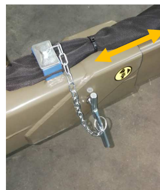
Fig. 7.6-2 - Extension stopping pin of an outrigger
