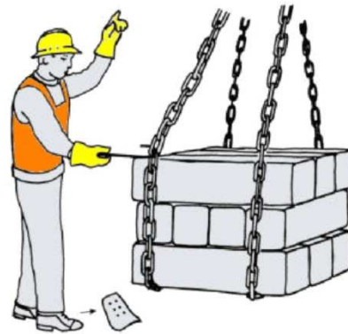
Fig. 5.3-8 - Suspended load guided with a hook
