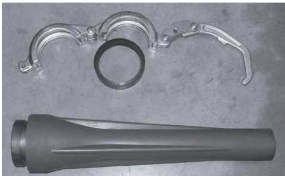
Fig. 7.10-1 - Nozzle disassembled in its parts
