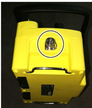
Fig. 7.4-4 - Connection plug via cable (closed with cap) of the remote control pushbutton panel
