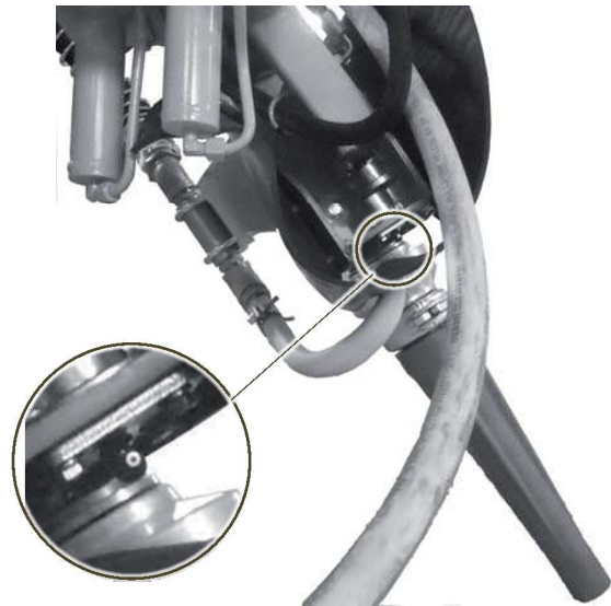
Fig. 8.14-2 - Nozzle holding wrist lubrication points
