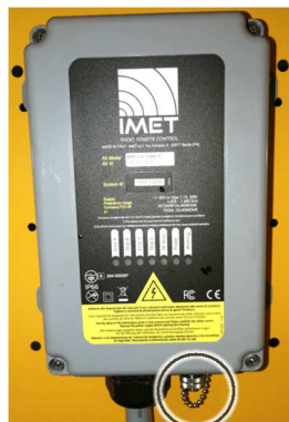
Fig. 7.4-5 - Remote control with connection plug in the lower part
