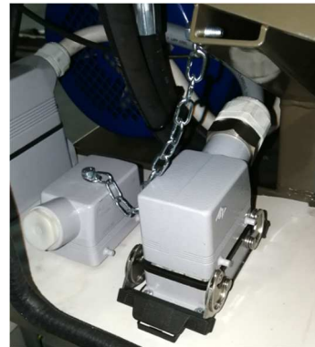
Fig. 7.4-3 - ILME socket inserted into the “IM2” plug of the electric control board for machine operation with radio control
